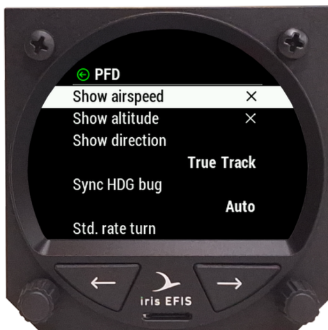
Figure 8. "Show airspeed", "Show altitude", "Show direction" options in setup page, Display and Graphic, PFD menu
