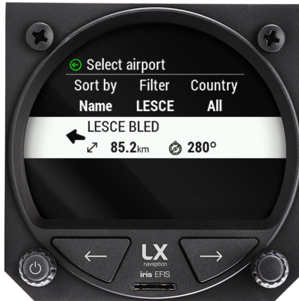
Figure 46. Scroll down and select the desired APT
