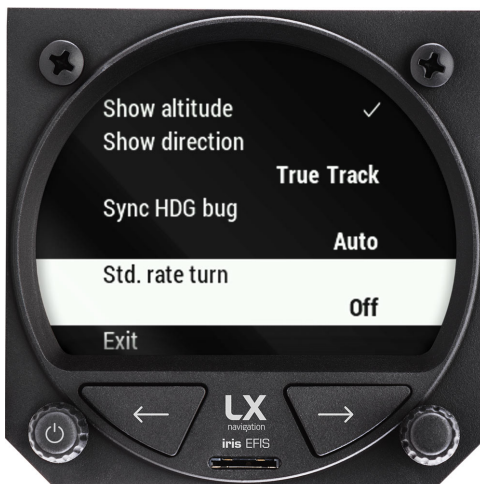
Figure 18. Standard rate turn indicator settings
