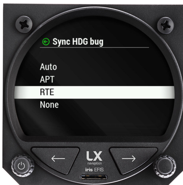
Figure 23. Magnetic heading bug - Sync function options
