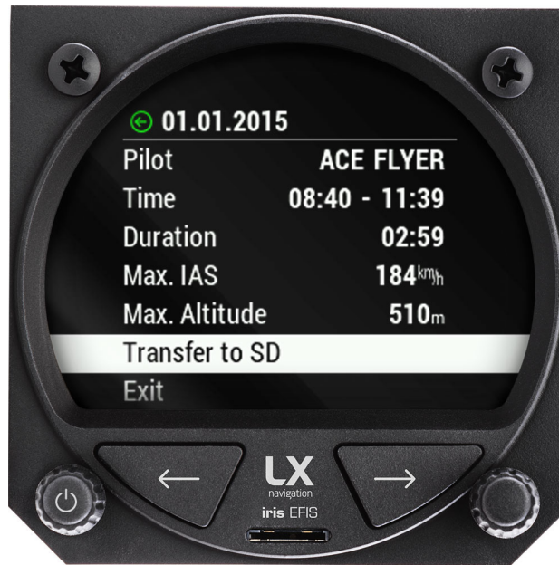
Figure 73. "Flight details" page with flight details and "Transfer to SD" option
