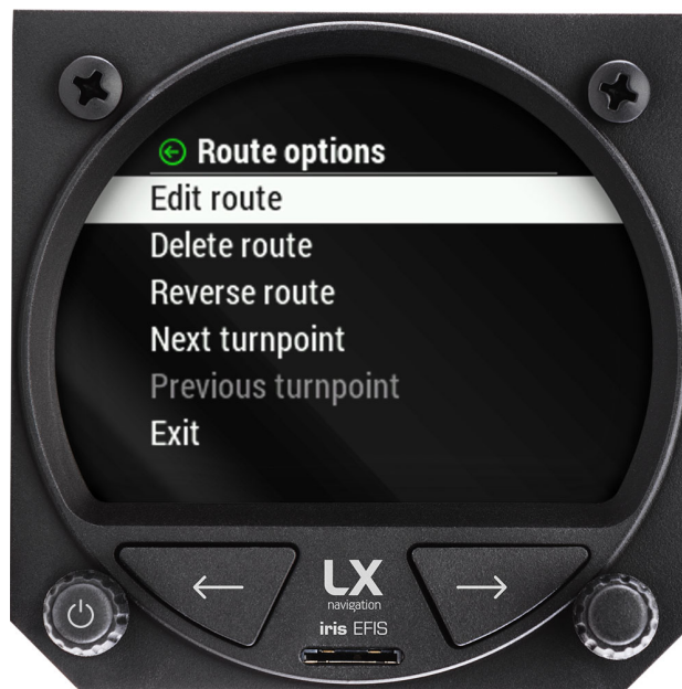
Figure 63. route options menu accessible - push left-hand push-rotary knob while at RTE page
