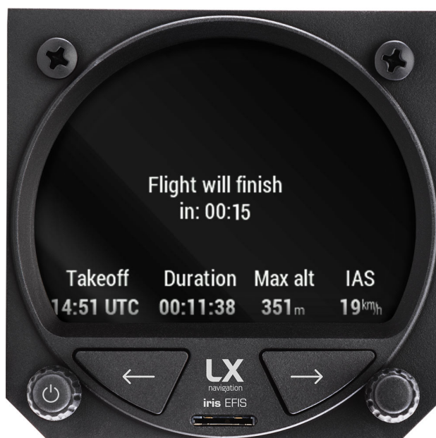
Figure 77. Device will end flight automatically after the airspeed and altitude is "0".
