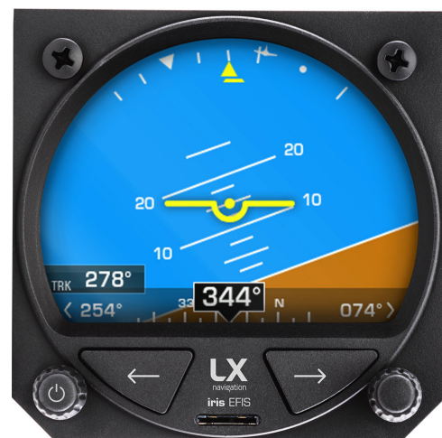
Figure 13. "Show airspeed" and "Show altitude" are disabled and "Show direction" is set to "True Track"
