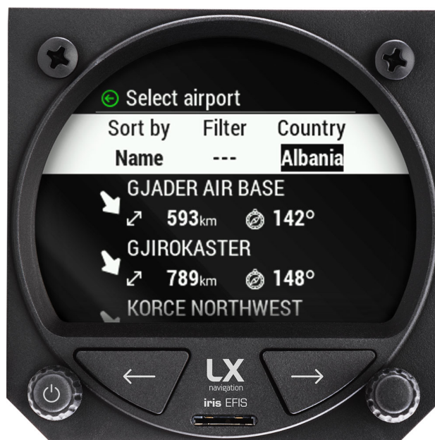
Figure 45. Adding "Country" parameter with rotating right-hand push-rotary knob
