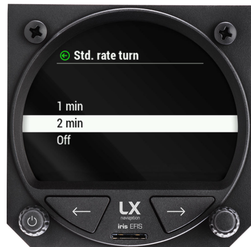
Figure 19. Standard rate turn indicator options
