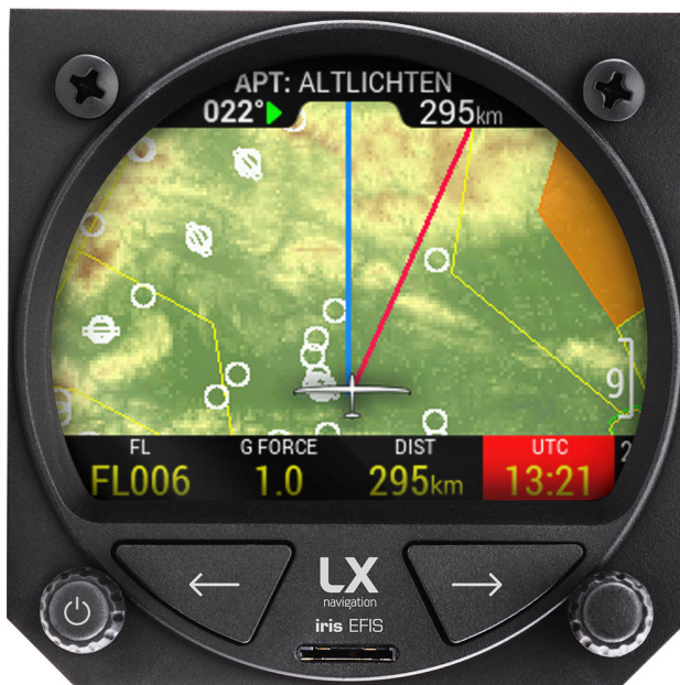
Figure 40. Press and hold the right-hand push-rotary knob to edit NavBox
