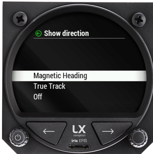
Figure 22. Direction tape bug - Show direction options
