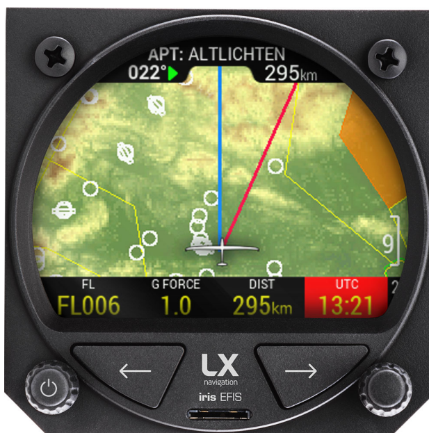
Figure 55. Press and hold the right-hand push-rotary knob to edit NavBox
