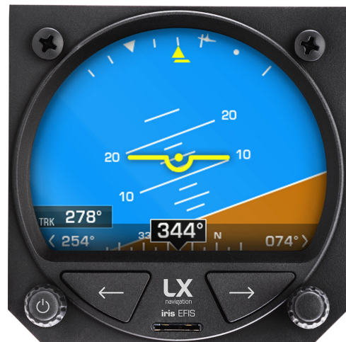
Figure 9. "Show airspeed" and "Show altitude" are disabled and "Show direction" is set to "True Track"
