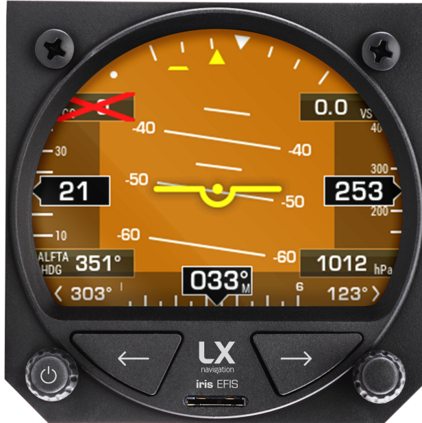
Figure 7. No Ground speed (GS) means there is a problem with GPS
