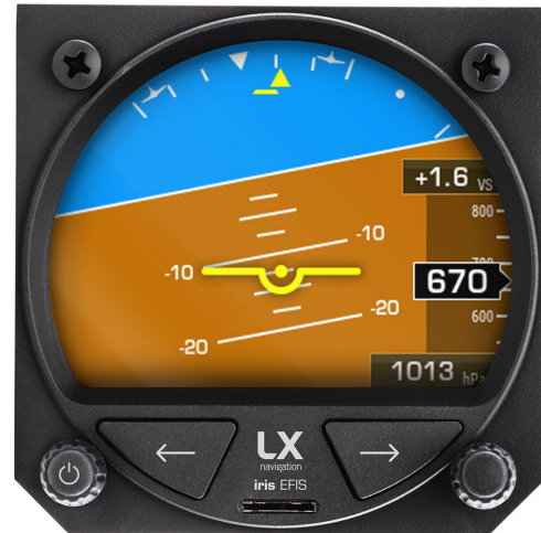
Figure 11. "Show airspeed" and "Show direction" are disabled, "Show altitude" is enabled
