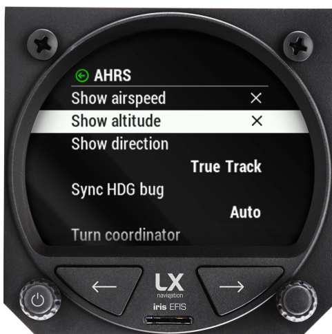
Figure 12. "Show airspeed", "Show altitude", "Show direction" options in setup page, graphic, PFD menu
