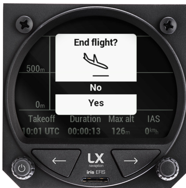
Figure 76. Manually "End flight" by pressing right-hand push-rotary knob while on Statistics page.
