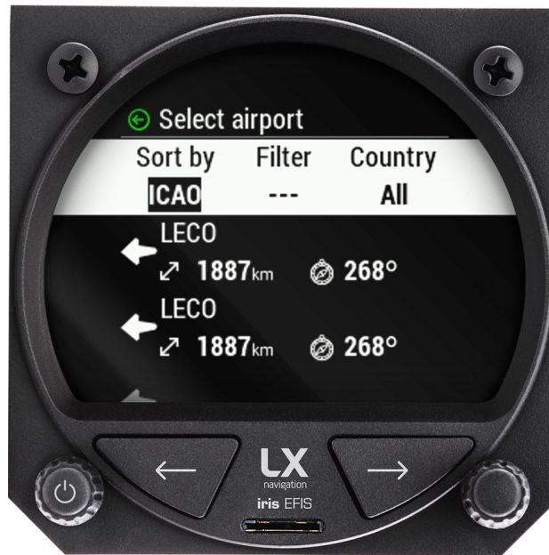
Figure 44. Adding "Filter" parameter with alphanumerical value
