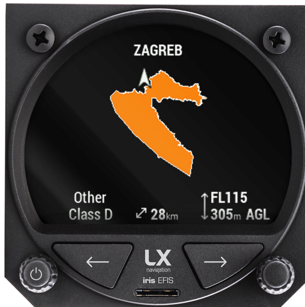
Figure 81. Airspace details page with graphical representation of airspace
