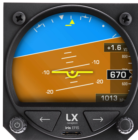
Figure 6. "Show airspeed" and "Show direction" are disabled, "Show altitude" is enabled
