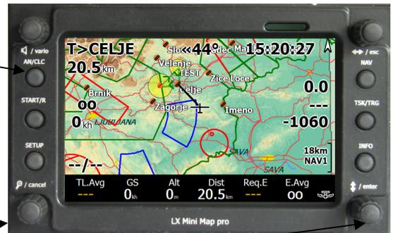
All **four rotary switches** also have a key function when pushed in.
