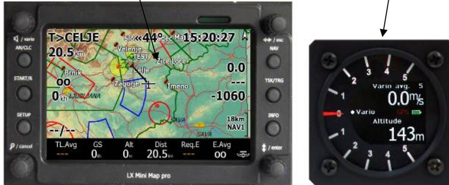
Both units are interconnected via LX Navigation system bus which enables both units to exchange data in both directions. The bus also powers the vario unit, thus the vario does not need a separate power supply.
