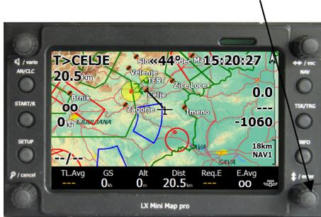
During navigation the key is used as a selector of navigation pages. In edit it is used as an up/down selector of items. Press will activate Enter function
