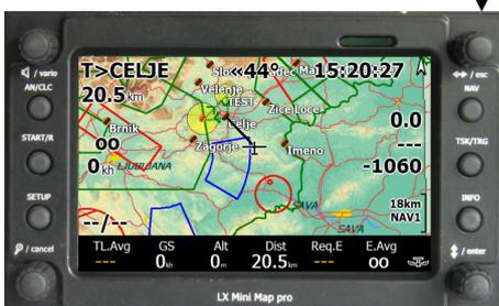
The main switch function is to rotate in - between bottom row pages (1-9) in basic navigation page (map) and to select horizontal sub pages. (See also further instructions that follow). The switch also selects in setup.
