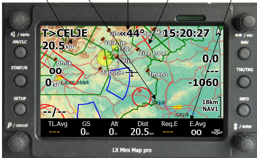
**Terrain** : terrain in different configurations as a background (see setup **1site** about details)
