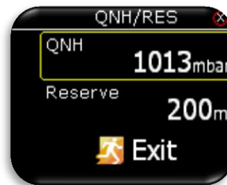
Value can be changed with rotary switch (yellow frame).
