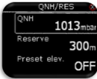
Pilot should set actual QNH and elevation of the airport where he will take-off on initial setup screen. After change of QNH during flight, pilot can change altitude information to which final glide will calculate. If QNH is changed on the ground, altitude will not be corrected and will still be the same as set on initial setup.
