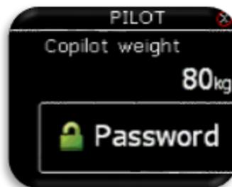
Co-pilot's weight is added to the whole weight of the plane.
