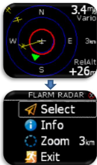
The graphic display is divided into 2 or 3 circles (depends on zoom setting). Last circle represents zoom distance. The white glider symbol is always positioned in the middle of the screen and shows the current position of the plane.
