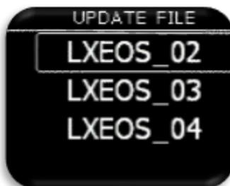
Pilot should copy new version to **root** of external micro SD card, then insert it into the LX Eos and use "Update" option to make an update of the unit. After selecting "Update", list of all version (\*.lxu) files will be listed. Pilot should select version, which he wishes to update to.
