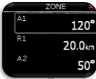
User can change A1, R1, A2, R2, zone type, A21 and auto next option. If auto next option is enabled, next TP is automatically selected, when pilot reaches TP zone.
