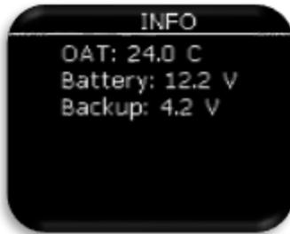
OAT and battery voltage levels are shown here as alphanumeric values.
