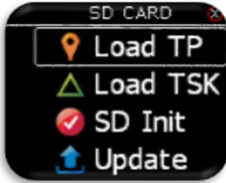
External SD card is used for all data transfers to LX Eos. In this menu all import/load functions from SD card can be accessed.
