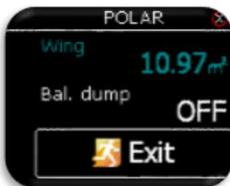
With ballast dump setting, pilot can set how many kg/min will be dropped out when using ballast switch on ballast valve. With this setting, ballast will be automatically reduced when valve is opened.
