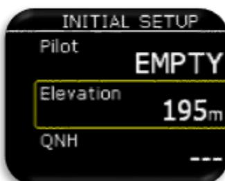
Select pilot from the internal database with rotary switch. If there is no pilot in database, "Empty" pilot is offered and can be later edited (name, surname,...) in Setup/Pilot menu. Code input will be required if selected user has his profile protected with user code.
