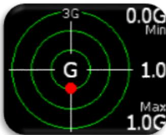
During the flight red dot of G-force page is showing current detected G-force. On right top and bottom corners, minimal and maximal detected G-force during the flight are displayed. This values can be cleared anytime during the flight in G-FORCE menu. In the middle, current G-force value is displayed. Range setting is presented with small text on top of G-force scale (example is showing 3G range). This range can also be set in G-FORCE menu.
