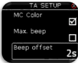
Thermal assistant page can assist pilot when thermaling to get better sense how thermal looks like. Thermal is presented with use of different coloured dots.
