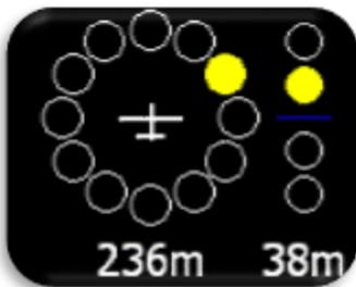
When flarm warning is detected, Eos will show Flarm warning page with direction, above/bellow indicator and numerical information for distance and relative altitude.
