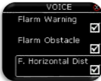
Enabling Flarm warning option will generate voice warning when Flarm collision warning is detected.
