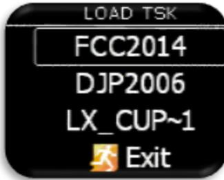
After selecting "Load TSK" option, list of all CUP files (up to 20) found on external SD card in LX/TP folder will be listed here. Select file from which you wish to import TSK to internal memory.
