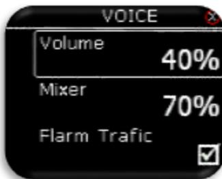
Pilot can set the voice volume of the device and mixer settings. The percentage of mixer means how much voice is mixed with vario beep. Low percentage means lower voice to vario beep ratio and higher percentage means higher voice to vario beep ratio.
