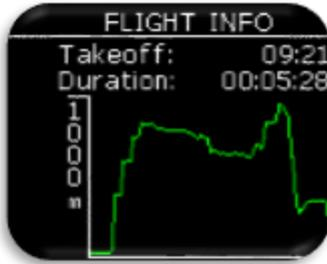
During flight, statistic of the flight is shown on statistic page. Take-off and duration time are displayed on top with baro altitude graph for last hour at the bottom.
