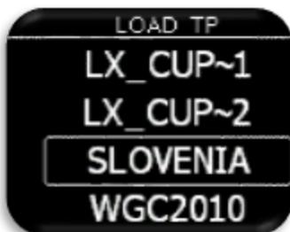
After selecting "Load TP" option, list of all CUP files (up to 20) found on external SD card in LX/TP folder will be listed here. Select file from which you wish to import TPs to internal database.
