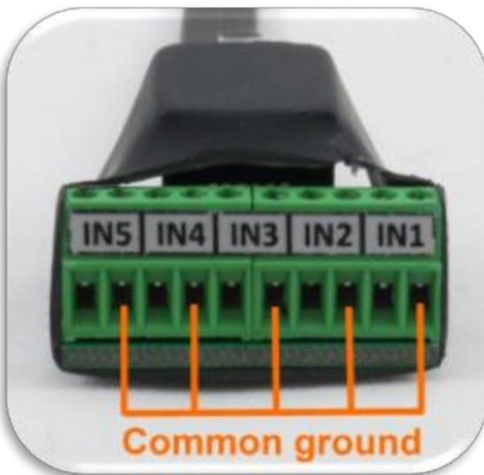
Up to five external switches can be connected to LX Eos. To connect external switch to LX Eos you have to use external switch interface board (included in package). Every slot available has a signal input and ground input. The configuration of inputs can be set under Setup -> Inputs.
