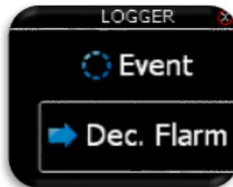
Dec. Flarm: Send declaration on Flarm port. If connected to Zeus, this is done automatically.
