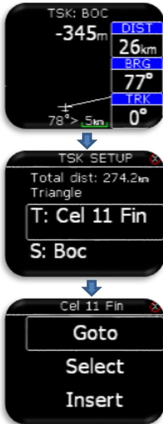
On the top of this page pilot can find name of navigated TP. Under the name, final glide to the end of the task is displayed. Navbox-es shows track (TRK), bearing (BRG) and distance (DIST) to the navigated point. Under the plane, steering symbol information will give pilot information for how many degrees (°) does he need to correct his track to fly directly to the point.
