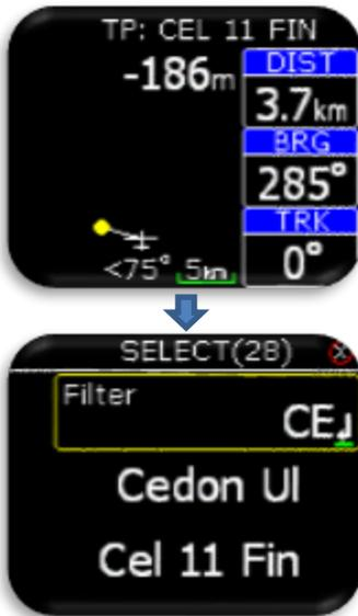
On the top of this page pilot can find name of navigated TP. Under the name, final glide information to the selected point is visible. Final glide calculates reserve altitude into end result. Navbox-es shows track (TRK), bearing (BRG) and distance (DIST) to the selected point. Under the plane, steering symbol information will give pilot information for how many degrees (°) does he need to correct his track to fly directly to the point.
