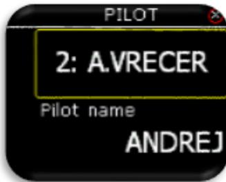
Pilot can either select pilot that is already saved in the database or select "EMPTY" to create a new pilot. If pilot is already saved, name initial and surname are shown. Pilot name or "EMPTY" is automatically shown in the second line. Code input will be required if selected user has his profile protected with user code.
