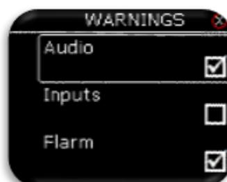
Pilot can enable (box is checked) audio warnings and Flarm warnings.
