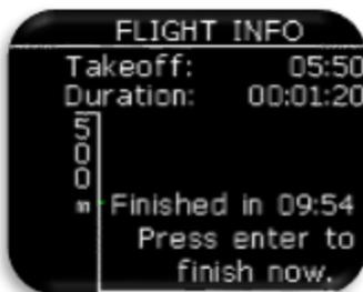
After pilot has landed, flight recorder will start 10min countdown, before flight will be automatically finished. This page will be shown automatically after 10s of countdown to alert pilot that flight will end after 10min. Pilot can wait until countdown or press enter to end flight immediately.
